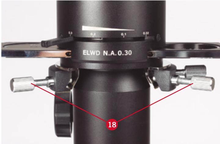
Those 2 diagonal screws on the front side of the condenser carrier (18) help to center the light spot, means the illumination in general. Move them until the light spot is placed in the middle of the image (19). Open the Field diaphragm until the complete field is illuminated (20).
