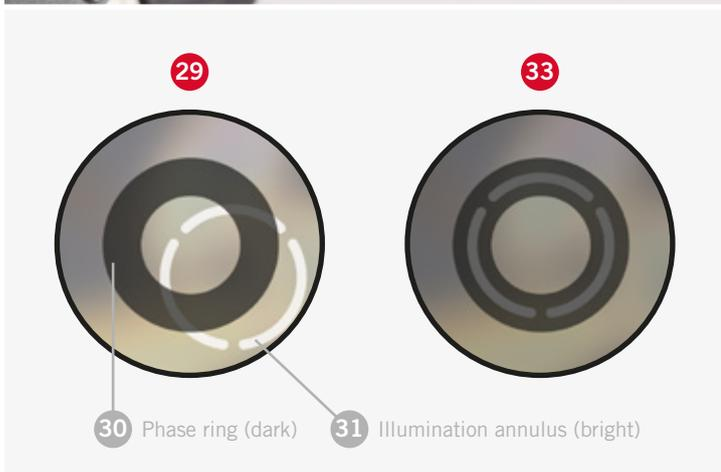
*Attention: This focussing procedure must be done by moving the inner part of the Centering telescope. Please do not touch the coarse/fine focus knobs.*
