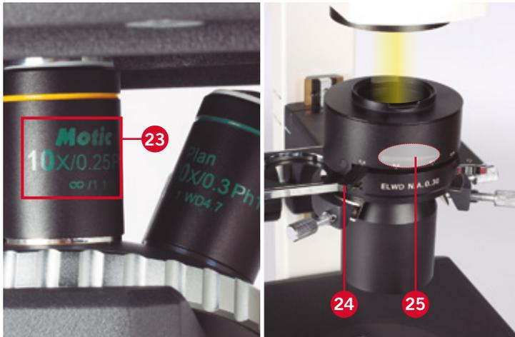
All Phase contrast objectives can be recognized by their GREEN labelling (international standard) (23). The code Ph0, Ph1, etc. refers to the physical ring size. All Phase objectives can also be used (with minor restrictions) in Brightfield.
