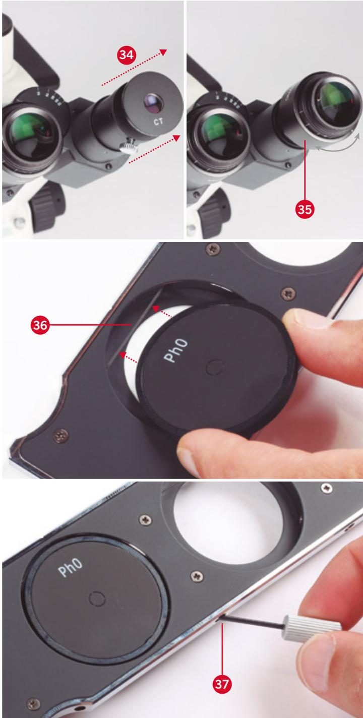
As the Ph1 ring size fits to the objectives 10X/20X/40X, the alignment is done for these objectives. In case of 4X objective lens, the appropriate annulus has to be aligned accordingly using the Ph0 ring. Pull out the Centering telescope (34), push in the eyepiece with a rotating movement (35). If the image of the illumination ring is diverging from the Phase plate in the objective, a low phase contrast image, similar to an oblique illumination, will result.
